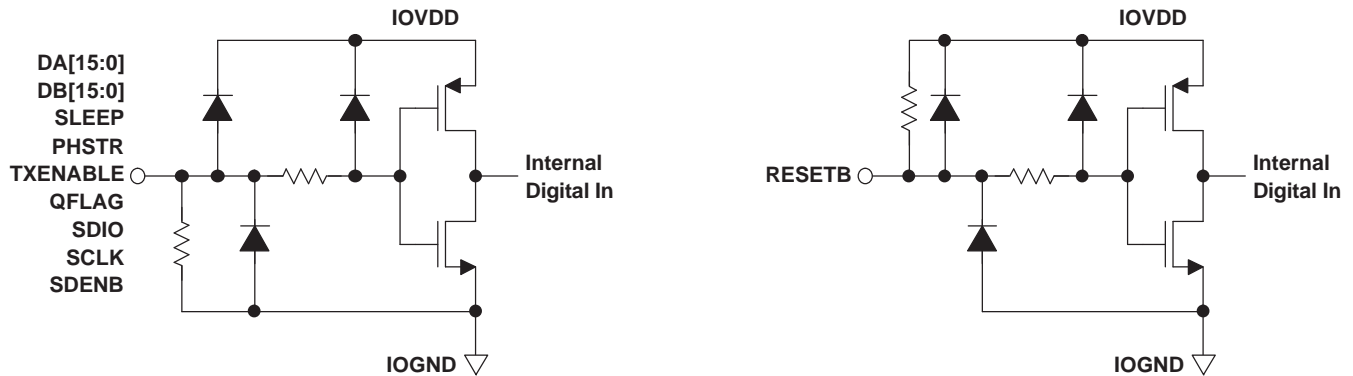
Figure 63. CMOS/TTL Digital Equivalent Input
